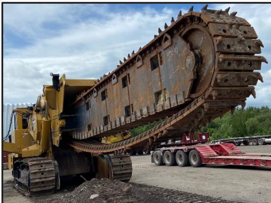
Trencor rock trencher to be used for bedrock excavation
